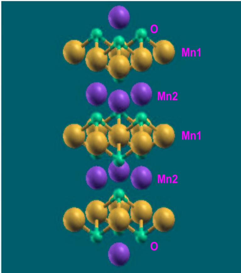
B1 structure with Mn moments aligned ferromagnetically in the [111] plane, with adjacent sheets having antiparallel spin
