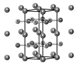
Fig. 1. Crystal structure of LiBC. The graphene structure of the B–C layers is a direct generalization of the B layers of  $MgB_2$ , and the Li atoms reside on the Mg site of  $MgB_2$ . The unit cell contains two formula units because B and C alternate in position along the  $\hat{c}$ -axis (i.e. the two B–C layers are connected by a  $120^{\circ}$  screw axis).
