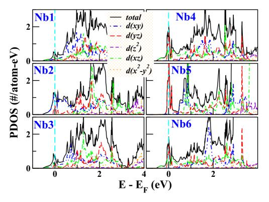
FIG. 2. (Color online) Total and orbital-projected density of states for each of the Nb sites in nonmagnetic  $Nb_{12}O_{29}$ . Note that Nb5 dominates the peak at the Fermi level  $E_F$ , while Nb2 dominates the occupied states at and below  $E_F$ .
