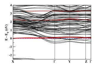
FIG. 3. (Color online) Full band region of nonmagnetic Nb<sub>12</sub>O<sub>29</sub>, above the gap separating them from the O 2*p* bands. The red horizontal lines indicate a single, remarkably flat,  $d_{yz}$  bonding and (split apart) antibonding band pair of the Nb5<sub>2</sub> dimer. Symmetry points are  $X = (\frac{\pi}{a}, 0, 0)$ ,  $Y = (0, \frac{\pi}{b}, 0)$ , and  $Z = (0, 0, \frac{\pi}{c})$ .
