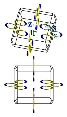
FIG. 3. (Color online) NbP Fermi surfaces (FSs) including SOC and shown from two angles, the lower one viewed along the  $k_x$  axis to reveal the thinness of the surfaces in the mirror planes. The extended zone representation makes the toroidal origin of the FSs evident. The hole (blue) boomerang FSs form bent and "sharply" tipped boomerang surfaces, the electron (yellow) new moon surfaces are similar but extend over a larger angle of the torus.
