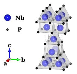
FIG. 1. (Color online) Body-centered-tetragonal  $I4_1md$  structure of NbP. It consists of edge-sharing NbP<sub>6</sub> trigonal prisms, which are  $90^{\circ}$  rotated in the next layer. The lack of inversion symmetry is evident: the prisms all "point" upward.
