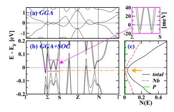
FIG. 2. (Color online) (a) GGA bands in the range of -1.5 to 1.5 eV and (b) GGA+SOC bands in the range of -0.2 to 0.2 eV, with  $E_F$  set to zero. The symmetry points can be identified in Fig. 3. The upper right panel enlargement shows the splitting by  $\sim 10$  meV of bands by SOC in this noncentrosymmetric structure. (c) Density of states (GGA+SOC) showing the pseudogap centered 20 meV below  $E_F$ .
