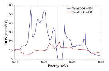
FIG. 3. Comparison of the density of states for ferromagnetic alignment (metallic) with that of the gapped nonmagnetic state, on a fine energy scale. The 13-meV gap is thoroughly washed out when magnetic moments are allowed to emerge and align.
