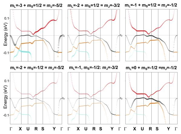
FIG. 6. The 5f fat-band structure of nonmagnetic UTe<sub>2</sub> from LDA+U(OP) calculations. The circle size indicates the amount of  $j=\frac{5}{2}$  and  $m_j$  character in the bands, as indicated. The two contributions to the  $j_z=-\frac{5}{2}$  character are quite different; the differences in the other two cases is are not so pronounced. Note that the full energy range is only 300 meV.
