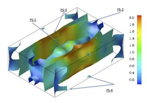
FIG. 5. Fermi surface for FM order, from LSDA+U(OP), centered at the  $\Gamma$  point. The Fermi surface is large and multisheeted, with a nesting feature for FS-3 near  $(0, \frac{\pi}{b}, 0)$ . FS-1 is in the center; FS-2 parallels FS-3 along parts of its length. The low velocities, given by the colorbar, extend over at least an order of magnitude, up to nearly  $2 \text{ eV/Å} (\sim 2.5 \times 10^7 \text{ cm/s})$ .
