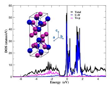
FIG. 1. Total and projected densities of states/eV (per unit cell) for nonmagnetic UTe<sub>2</sub> from the local spin density approximation plus Hubbard U [LSDA + U(OP)] functional, showing the total (black) and projections for U 5f (blue) and Te 5p (magenta). The Immm UTe<sub>2</sub> crystal structure is shown in the inset: blue spheres are U, and magenta spheres are Te. Note that the states near the Fermi level  $E_F = 0$  are entirely U 5f in character.
