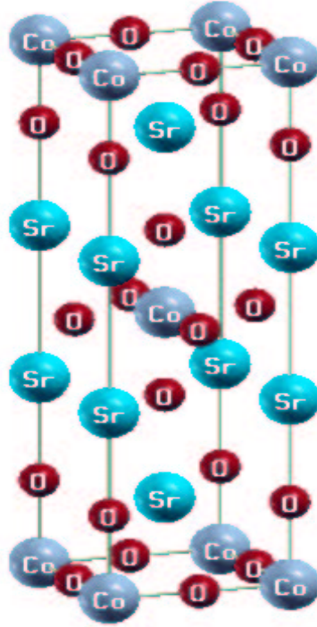
Figure 5.1. Crystal structure of \text{Sr}_2\text{CoO}_4 , a body-centered-tetragonal type. The planar O-Co bond length is 1.878 Å, about 6% shorter than the apical O-Co bond length. Lattice constants used here are a=3.755 Å and c=12.6 Å.
